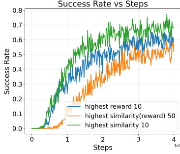
Figure 6. Success rate of residual RL trained with imitation priors from different K-means subsets. The "Highest Consistency 10" subset, despite having the lowest mean reward, achieves the highest success rate, demonstrating that trajectory consistency is the most critical factor for residual RL optimization.
